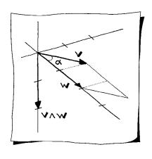
Area of parallelogram spanned by  ${\bf v}$  and  ${\bf w}$
