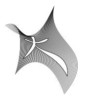
A Bézier surface trimmed by a ConS (Curve on a Surface)
