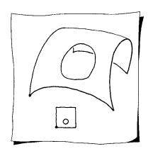
Parametric curve (u(t), v(t)) in the domain of surface  $\mathbf{x}(u, v)$
