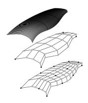
Top: bicubic B-spline surface Middle: B-spline control polygon Bottom: piecewise Bézier control net B-spline surface consists of a collection of individual polynomial patches
