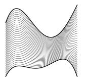
Application of the linear space properties of  $\mathcal{P}_n$  in shape design Feature curves (polynomials) designed over a common domain interval Shape formed from convex combinations of the feature curves Idea can be used for 3D surface design using the techniques in Chapter 20
