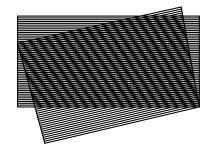
Two sets of parallel lines overlaid Interference pattern called *Moiré pattern*Used in optics for checking the properties of lenses
