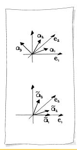
Shear/forward elimination concept provides an easy to visualize interpretation of the  $3 \times 3$  determinant
