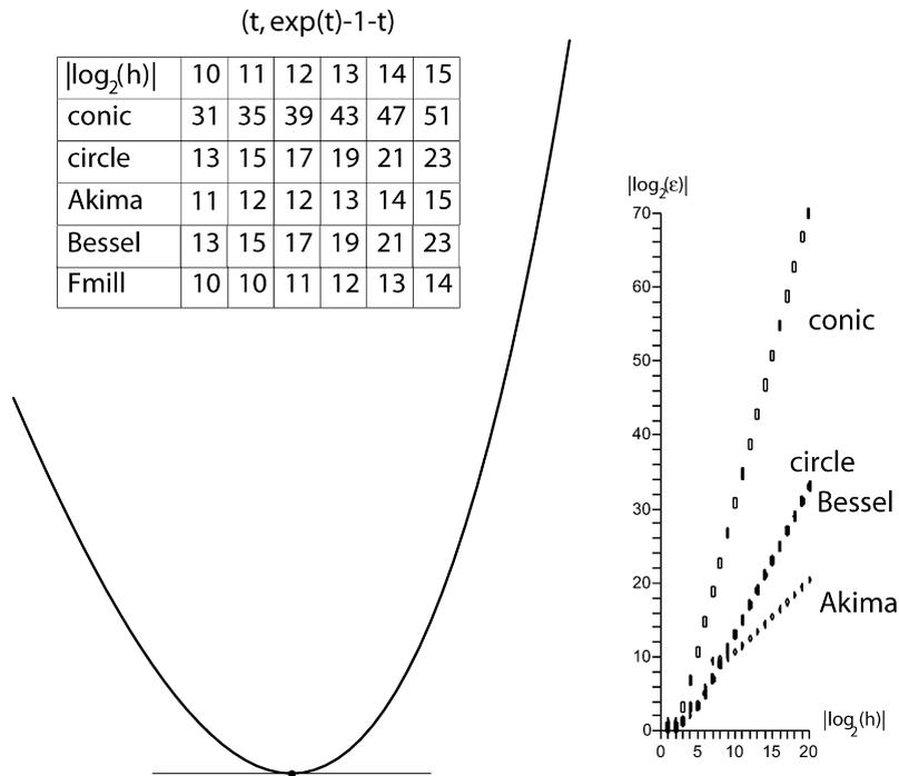
Fig. 6. Comparison of the tangent estimators for points taken from the curve  $(t, \exp(t) - t - 1)$ . The values of  $|\log_2(\epsilon)|$  for the different methods are shown in the table and partially illustrated in the graph.
