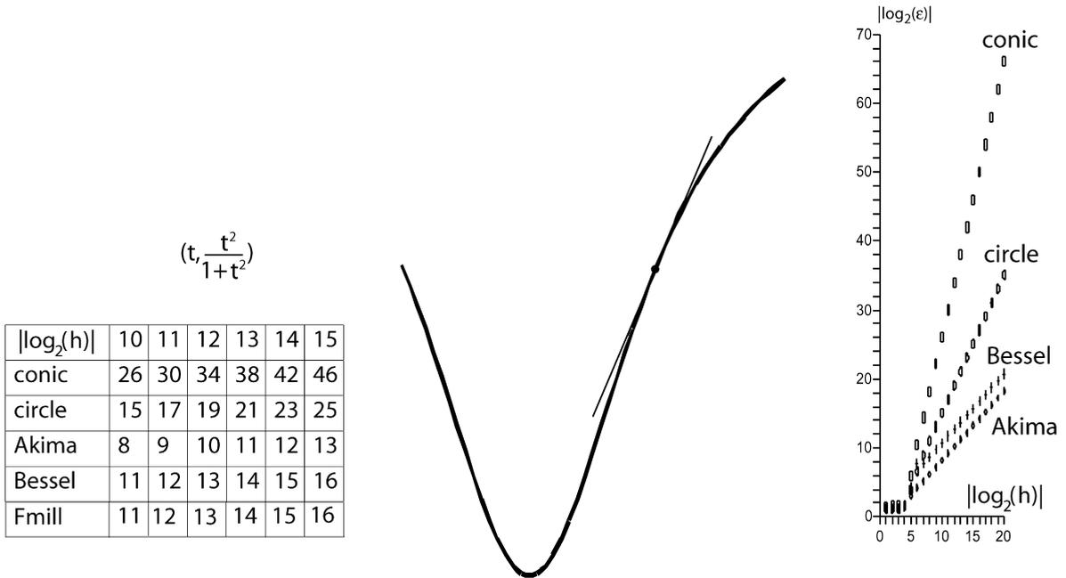
Fig. 8. Comparison of the tangent estimators for points taken from the curve  $(t, \frac{t^2}{1+t^2})$ . The values of  $|\log_2(\epsilon)|$  for the different methods are shown in the table and partially illustrated in the graph.
