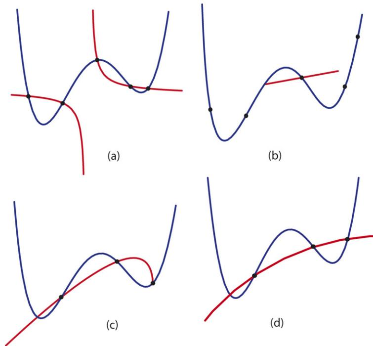
Fig. 5. Non-convex situation: erroneous tangents are obtained by the conic method (a) as tangent to the interpolating hyperbola at the middle point, by Akima's method (b), by Bessel's method (c) as tangent to the interpolating parabola at the middle point, and by the circle based method (d) as tangent to the interpolating circle at the middle point.
