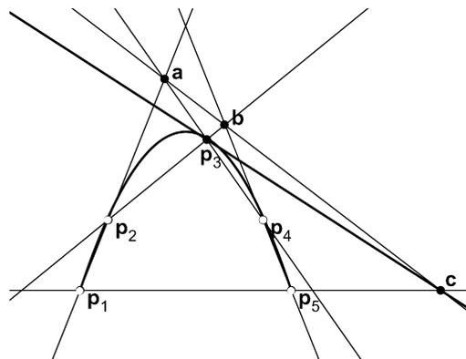
Fig. 2. Tangent construction: tangent  $\bar{L}_{33}$  at  $\bar{p}_3$  is formed using a special application of Pascal's theorem where two points have coalesced.
