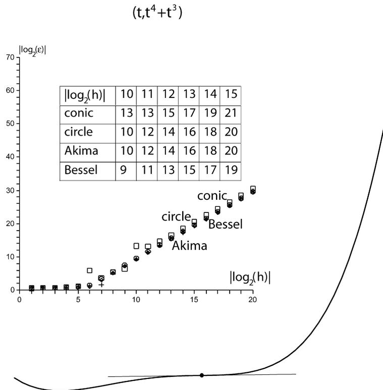
Fig. 7. Comparison of the tangent estimators for points taken from the curve  $(t, t^4 + t^3)$ . The values of  $|\log_2(\epsilon)|$  for the different methods are shown in the table and illustrated in the graph.
