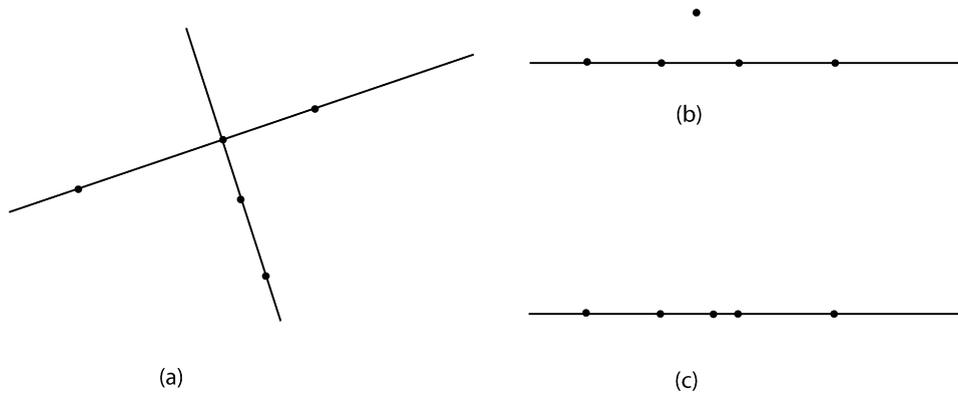
Fig. 3. Degenerate configurations, where the algorithm (6) produces an invalid result: (a) the conic degenerates into a pair of intersecting lines, where each of the lines contains 3 data points, the intersection point of the lines being a data point, (b) the conic degenerates into a pair of intersecting lines, where one of the lines contains 4 data points, (c) the conic degenerates into a double line containing all five data points.
