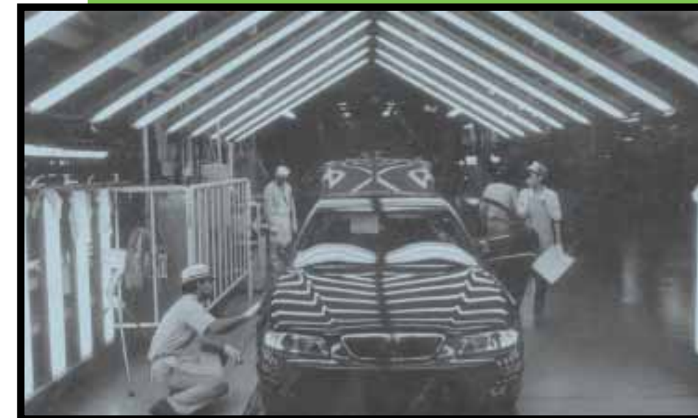
Figure 1. Real-life reflection lines used as a quality assurance tool.
